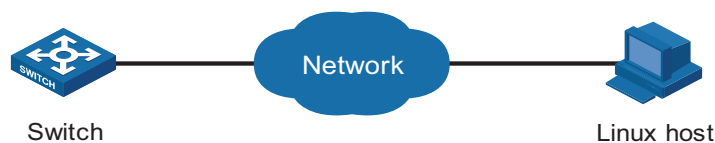
Figure 107 Network diagram for outputting log and trap information to a log host through the same channel
